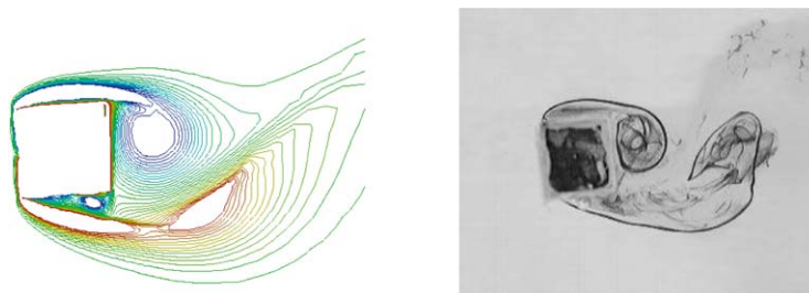
Fig. 17. Comparison between numerical and experimental flow visualization at Re = 1000 , \alpha = 4^\circ . No reattachment of the upper shear layer is seen.
